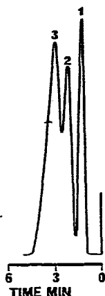
Fig. 1. Chromatogram of chlorpropamide (1), tolbutamide (2) and 1-isopentyl-3-( p -tolylsulphonyl)urea (3). Solvent system, acetonitrile—water (28:72, v/v).
